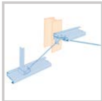
Diagonal Tie Wires
